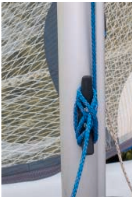
Picture 4.26 – the jib halyard cleat.
