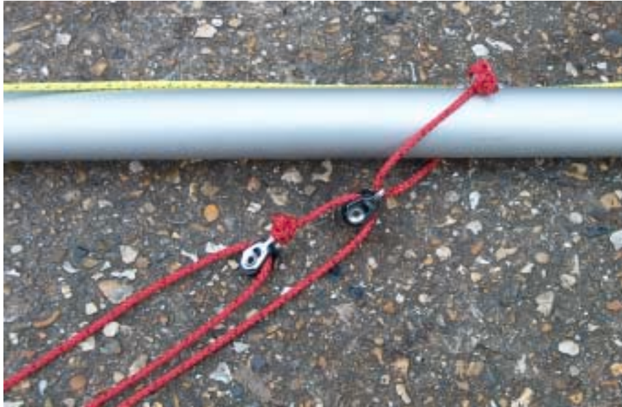
Picture 4.14 – the kicking strap attached.
