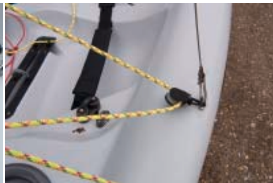
Picture 4.34 – the gennaker sheet block.
