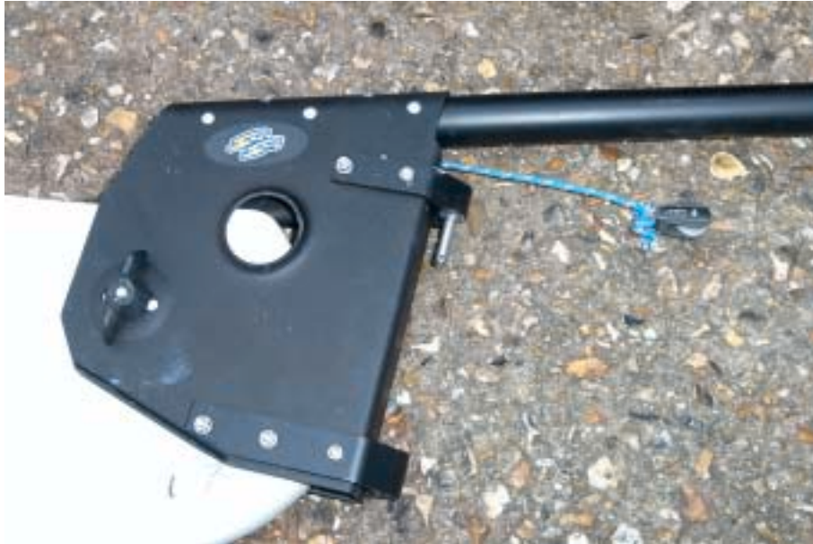
Picture 4.16 – the rudder fitted in the stock.
