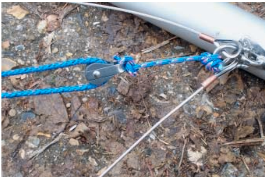
Picture 4.24 – fixing the jib halyard block.
