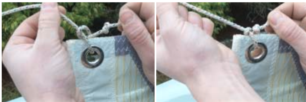
Picture 4.19 – tying the main halyard.
