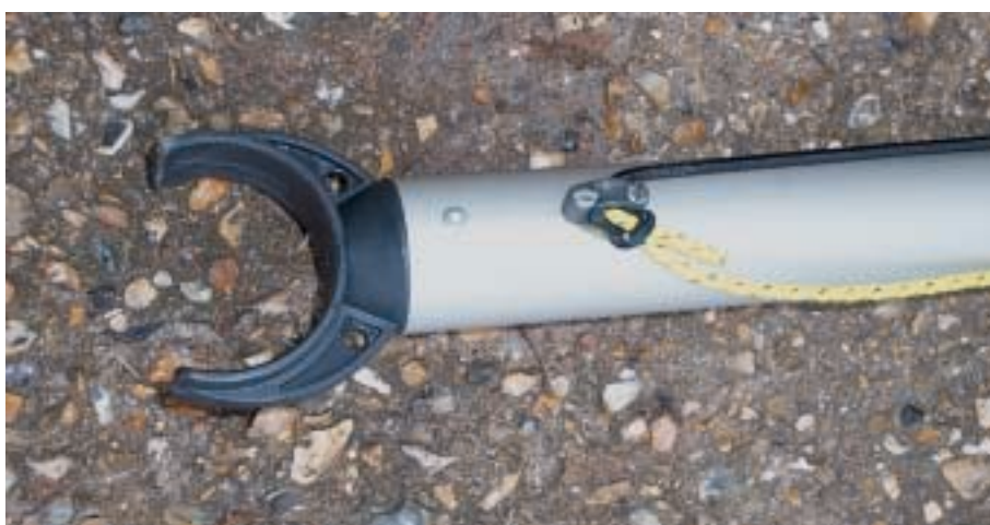
Picture 4.13 – the front end of the boom and gooseneck.
