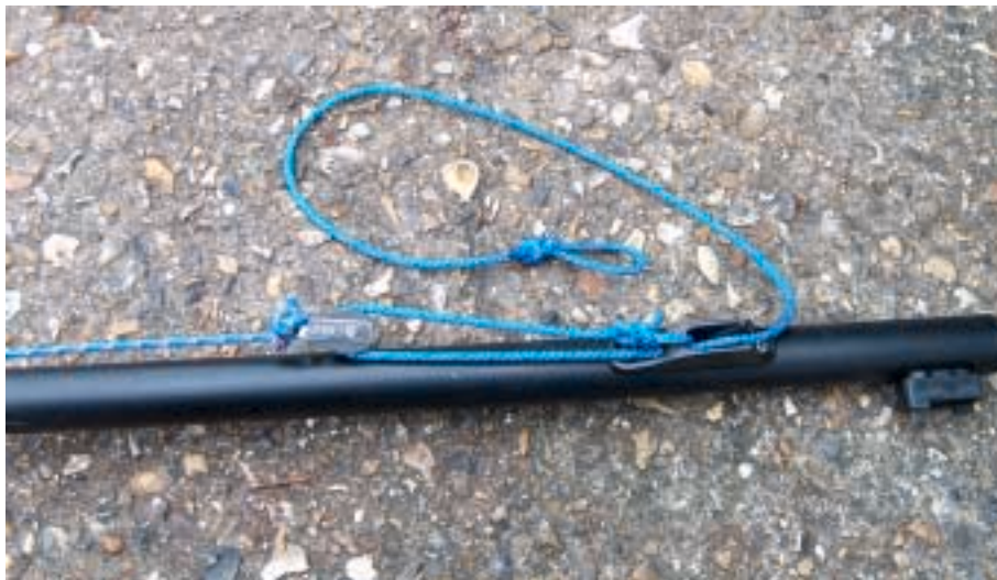
Picture 4.17 the rudder downhaul fitted.
