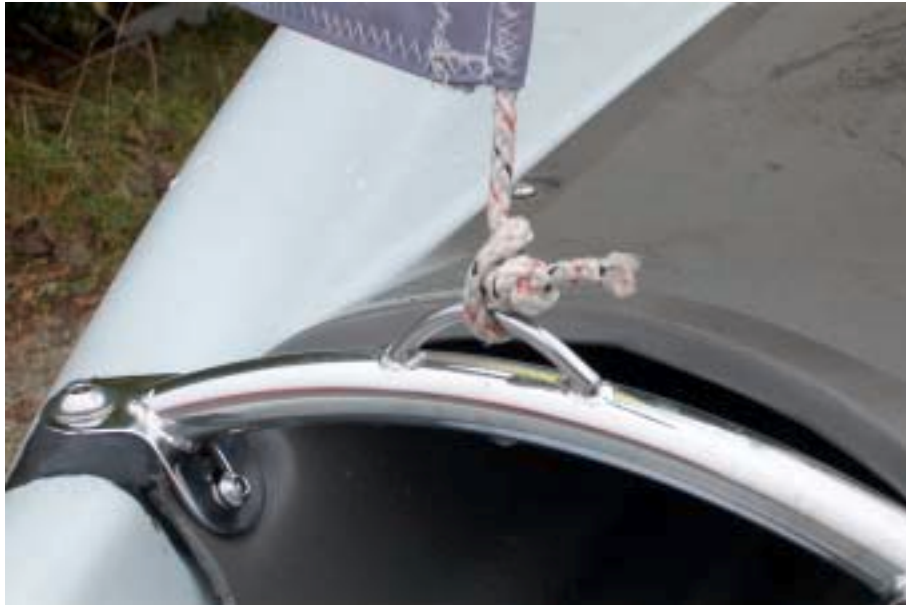
Picture 4.25 – the jib tied to the tack bar.
