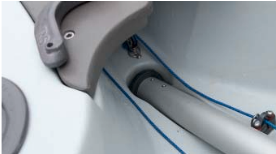
Picture 4.10 – the mast foot in the mast well.
