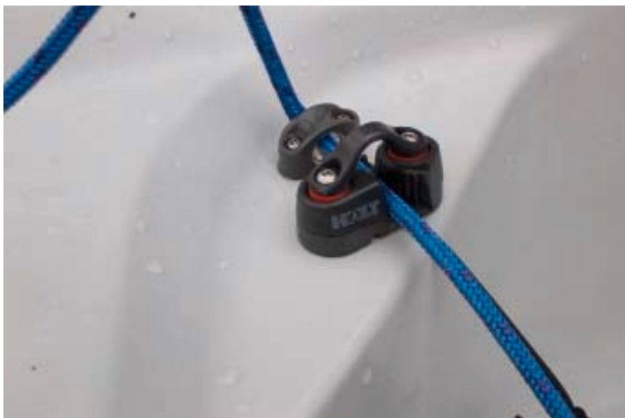
Picture 4.28 – the jib bullseye and cleat.
