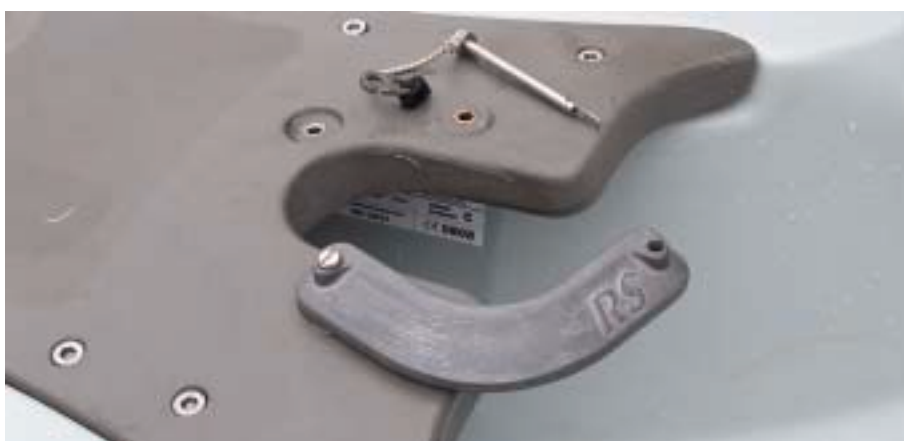
Picture 4.9 – the open mast gate.
