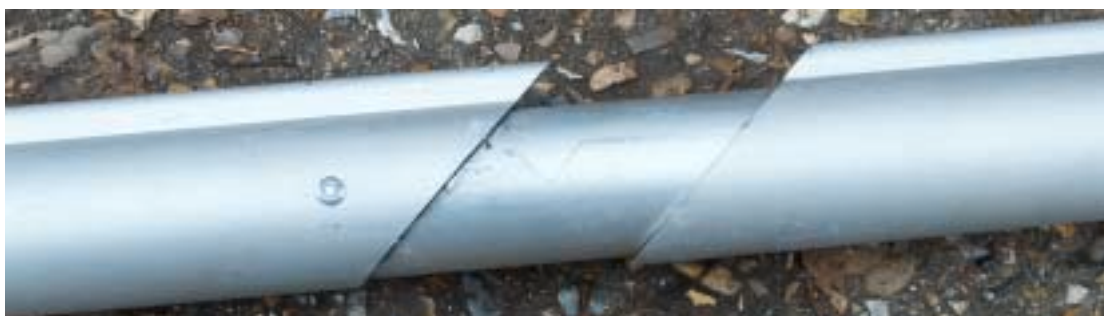
Picture 4.5 – joining the mast
