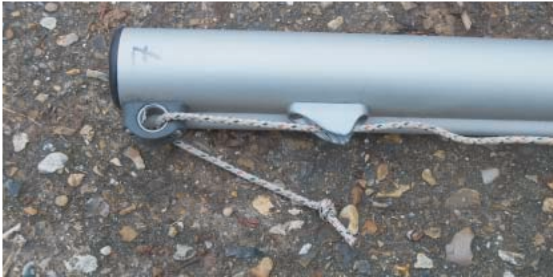
Picture 4.7 – threading the main halyard.
