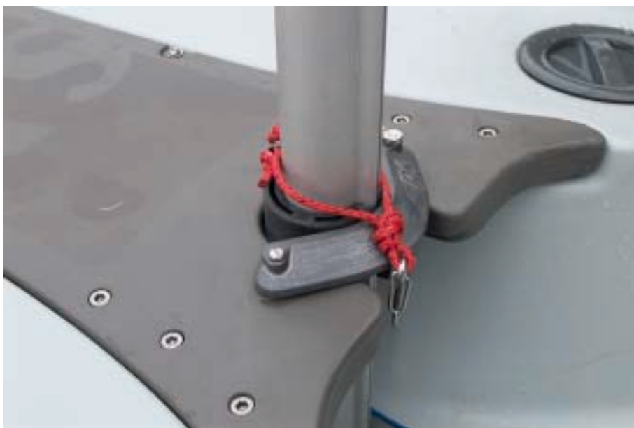
Picture 4.11 – the mast up with the gate closed.
