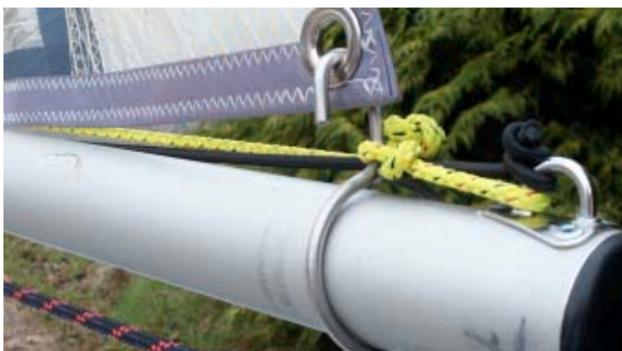
Picture 4.20 – the mainsail clew hook.
