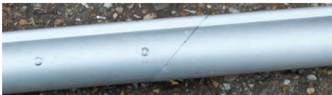
Picture 4.6 – a joined mast
