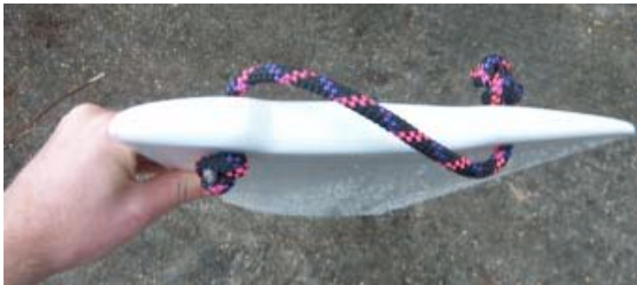
Picture 4.15 – the daggerboard handle.
