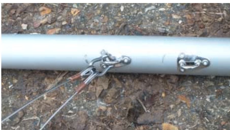
Picture 4.23 – fixing the shrouds.
