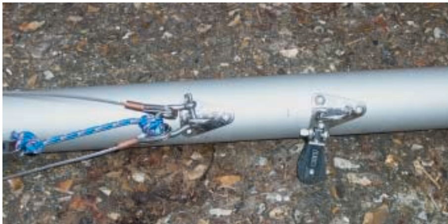
Picture 4.29 – the Gennaker halyard block.
